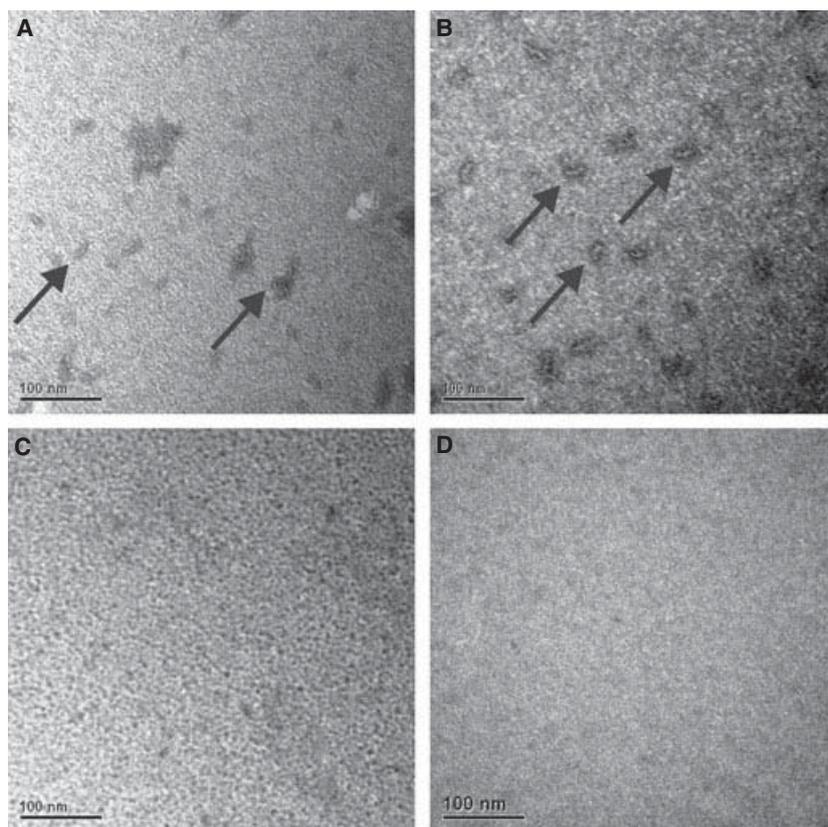
**Fig. 3.** TEM images of LLO in solution. (A) LLO at pH 5.5. (B) LLO at pH 5.5, preincubated at 37 °C for 30 min. Slightly curved particles visible at pH 5.5 are denoted by arrows. (C) LLO at pH 7.5. (D) Grid processed in the same way as in (A), (B) and (C), but without LLO.
